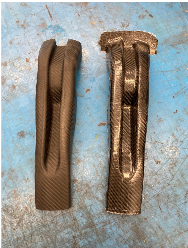
PAKT3D component and original component from the Ultem mould tool
