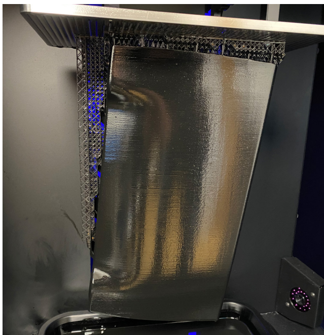
Automotive Interior Moulding. Print time under 6 hours
